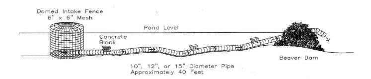
In order for these pipe systems to be effective, they must be designed so that beavers cannot detect the flow of water into the pipe. The Flexible Pond Leveler<sup>TM</sup> does this by surrounding the submerged intake of the pipe with a large cylinder of fencing which is placed in as deep water as possible. This prevents the beavers from detecting the flow of water into the pipe. As a result, the beavers do not try to clog the pipe, and a safe water level can be maintained.
