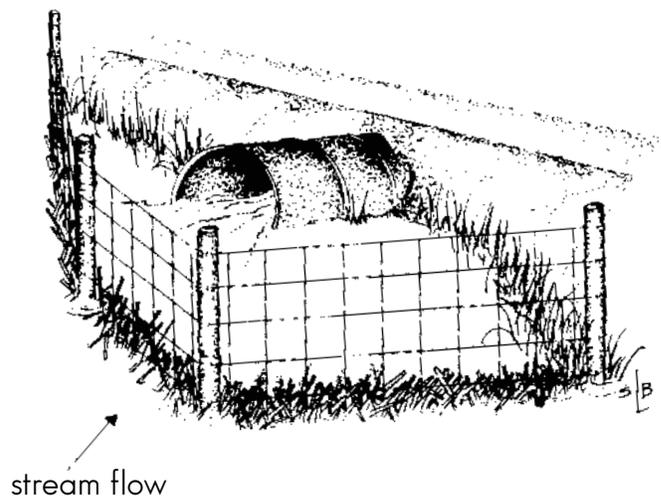
**Beaver Fence** Constructed on upstream side of a culvert, it keeps the culvert clear and allows high water to flow over dam and through the culvert.
