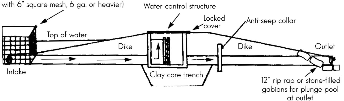
**Cross Section of Low Level Dike and Water Control Structure**
